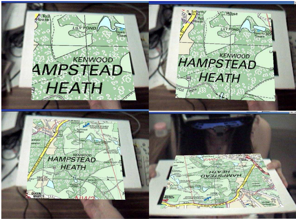
Figure 6.1: Different zooming of a 2D map. The user can draw the map close to the camera to view details as shown in the last image.
