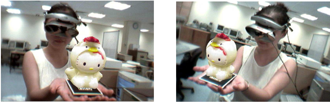
Figure 3.2: Different angles of 3D model attached to the marker viewed from head-mounted display(HMD)
