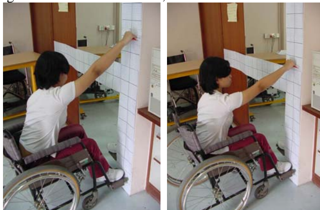
Figure A6.3: (Left) maximum up-forward reach to a wall. Figure A6.4: (Right) comfortable up-forward reach to a wall.
