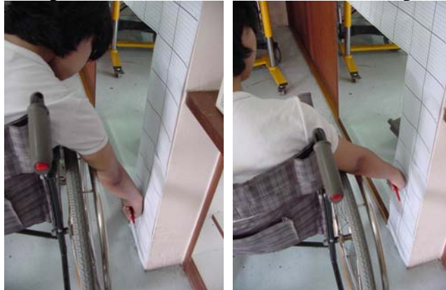
Figure A6.7: (Left) maximum downward reach laterally. Figure A6.8: (Right) comfortable downward reach laterally.
