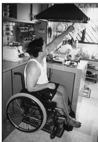
Figure A4. 15: Lowered hood was easy to reach.
