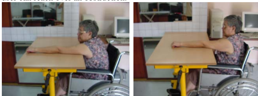
Figure A6.9: (Left) maximum forward reach over a table. Figure A6.10: (Right) comfortable forward reach over a table.
