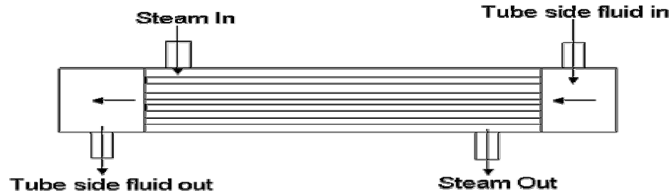
Figure 4.4.1: Simple Single-Pass Shell and Tube Heat Exchanger
