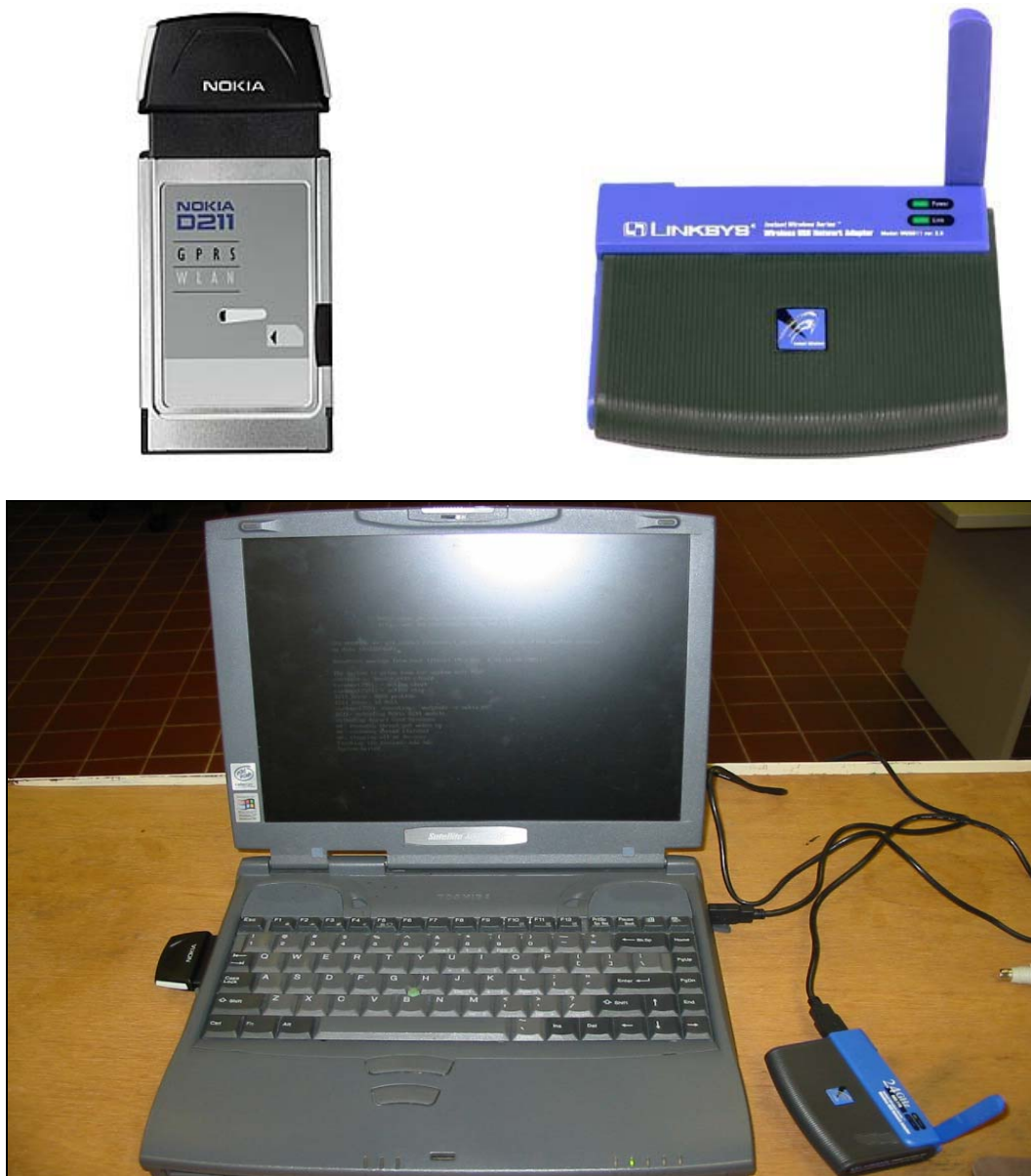
Figure 5.2 Mobile client with Nokia D211 GPRS PCMCIA modem (left) and Linksys USB WLAN network adaptor (right)
