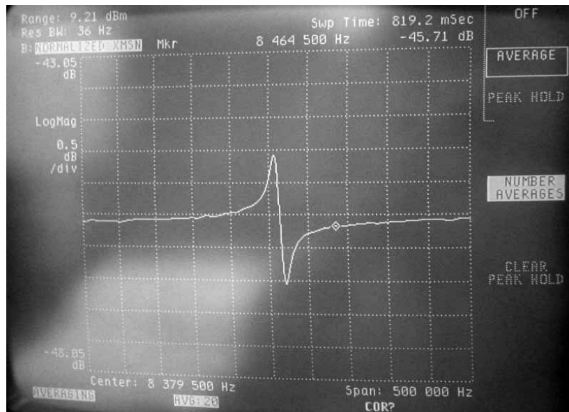
Figure 30. Measured frequency response of the micromechanical resonator (With 10 times of amplification).
