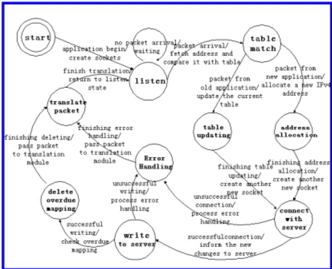
Figure 3.6. State transition diagram of client
