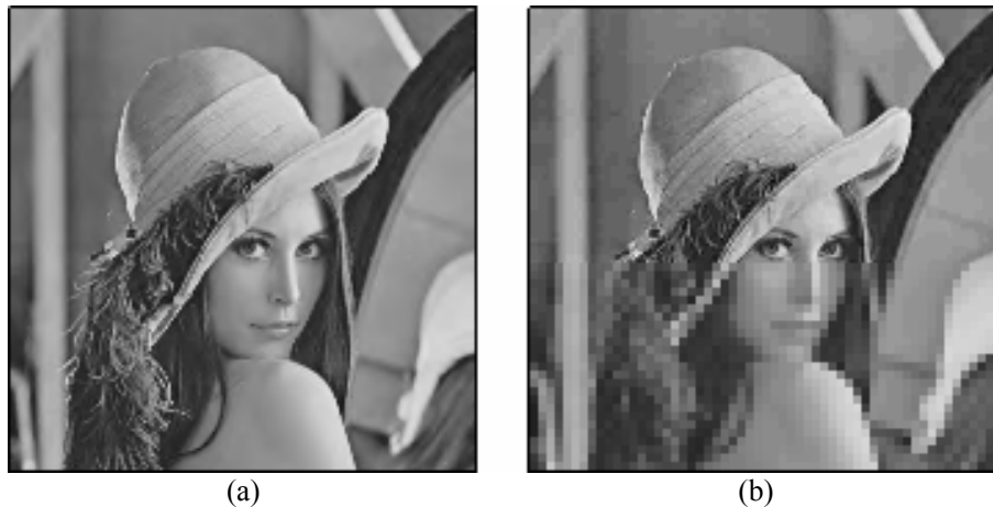
Figure 3-3 Lena reconstructed based on different schemes with the same rate (a)DWT + EZW. (b) Progressive JPEG
