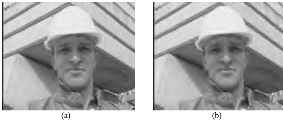
Figure 6-18 First frame (luminance) of foreman.qcif compressed at 0.5bpp by (a) SPIHT-FSOT with arithmetic coding and (b) JPEG2000
