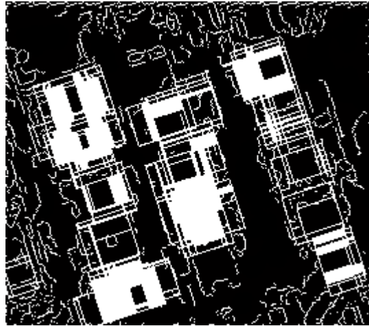
Fig. 4.25 Edge template matching – pixels 20 to 40 Accuracy parameter: 90%
