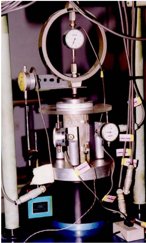
Plate 3.1 Apparatus for unconfined compression test with Hall's effect axial gage
