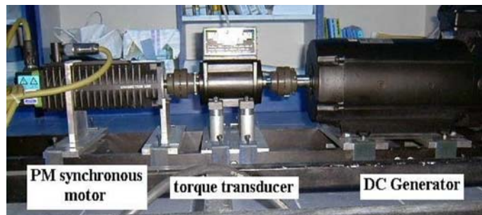
Figure 8.11. Configuration of DSP-based experimental setup
