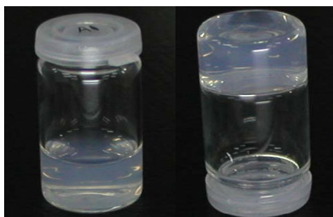
Figure 3-2. Photo images of C-F108 (1%) hydrogel sample at different position
