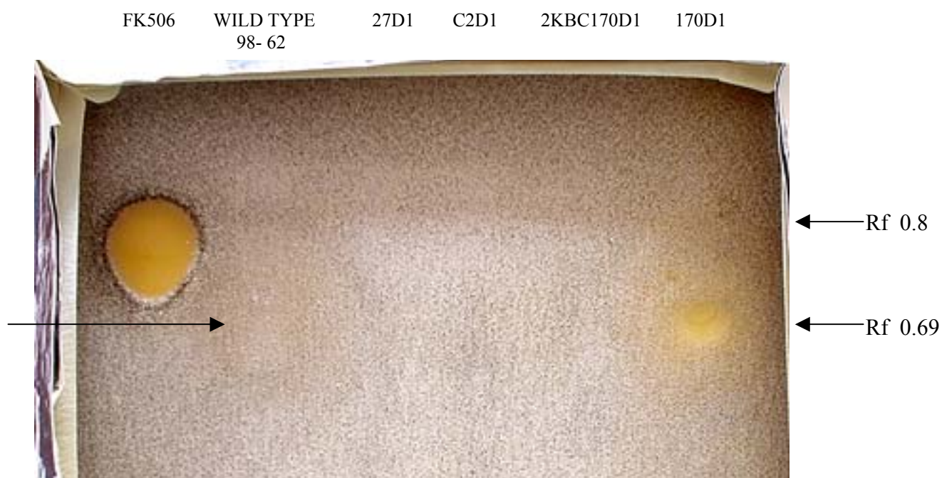
Figure 42: TLC chromatogram and overlay assay of the extracts of pure FK506, wild type Streptomyces sp. 98– 62, disruptants 27D1, 2KBC170D1, C2D1, C170D1. The cleared area represents the zone of inhibition. The test organism used was Aspergillus niger .
