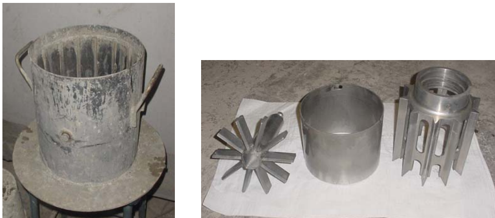
(b) Outer cylinder (container) and Inner cylinder (blades) used for Concrete Rheology test
