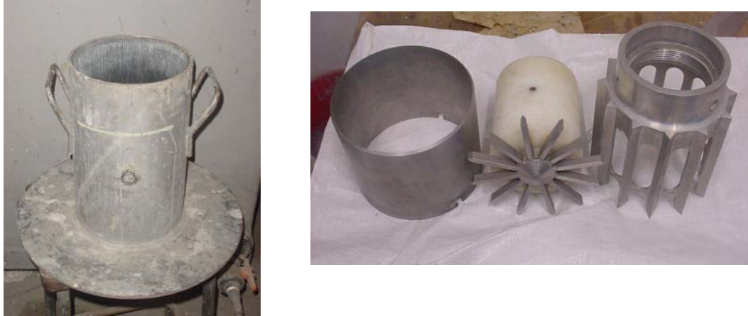
(b) Outer cylinder (container) and inner cylinder (blades) used for mortar rheology test
