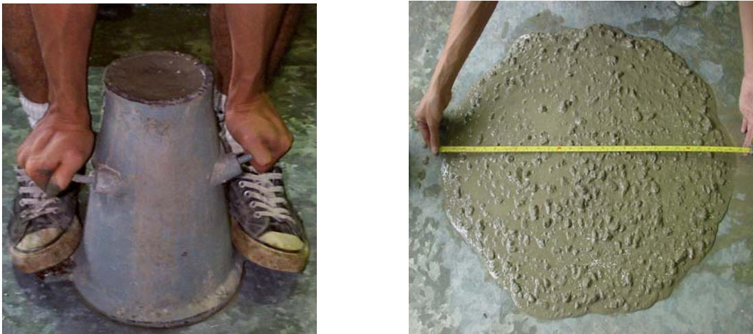
Fig. 8.5 Slump flow test and measurement of the ultimate slump flow diameter
