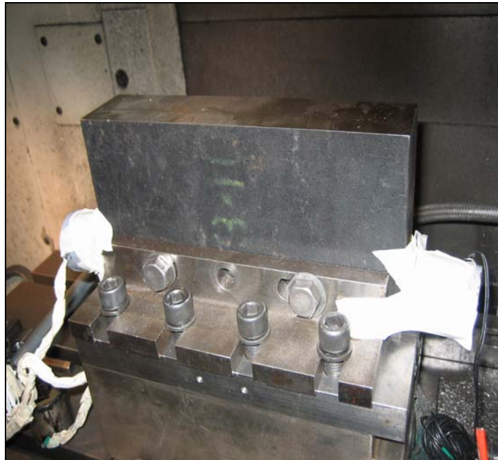
Figure 5.7 Electromagnets setup on workpiece in milling
