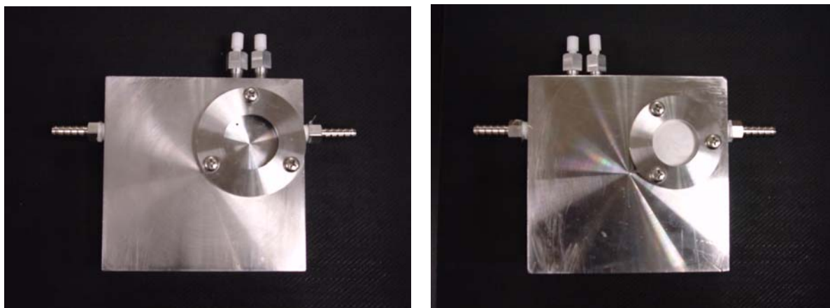
Figure 3.3. The left photograph is a close up of the liquid sample holder (without window present) and the right photograph is a close up of the solid sample holder (with polymer sample present).
