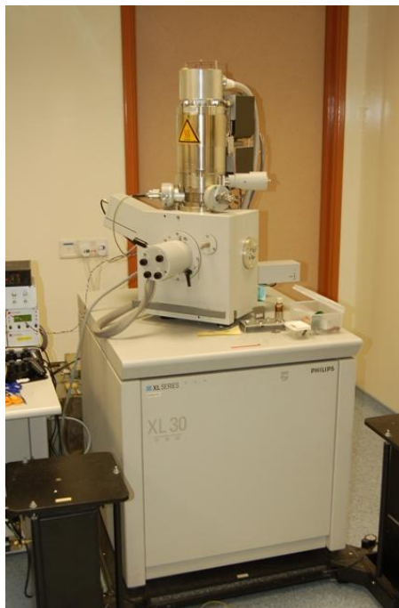
Fig 3. 7 Philips XL30 FEG scanning electron microscope
