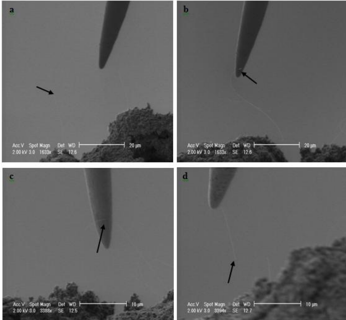
Fig 4. 3 Contacting between tungsten tip and CNT and pulling-out of CNT. (a) Long, straight and thin tube that is uniform in its diameter, points in the direction of the tip, and stands sufficiently free from other tubes to allow being approached (b) Free-standing end of the bent CNT sticks to the tungsten tip a few micrometers from the tip apex (c) CNT is aligned with the tip by pulling out the tube (d) Pulled-out CNT in the cantilever geometry with the new free end which is broken from the original tube indicated by black arrow
