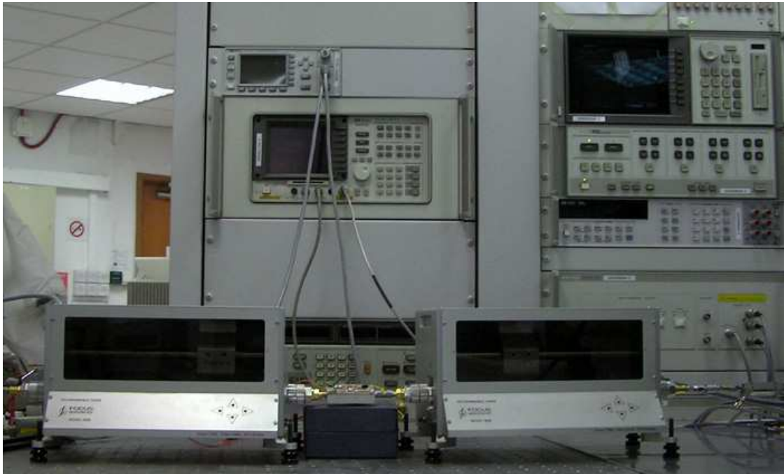
Figure 5.4: Load pull and source pull setup
