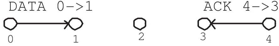
Figure 3.3: Two concurrent transmission in a 4-hop chain. The average interval T_d(4) between two consecutive packet transmissions from source node 0 is given by \sum_{i=0}^3 T_{Di,i+1} + \sum_{i=3}^1 T_{Ai,i-1} , where (i, i + 1) or (i, i - 1) means a packet is transmitted from node i to node i + 1 or to node (i - 1) .
