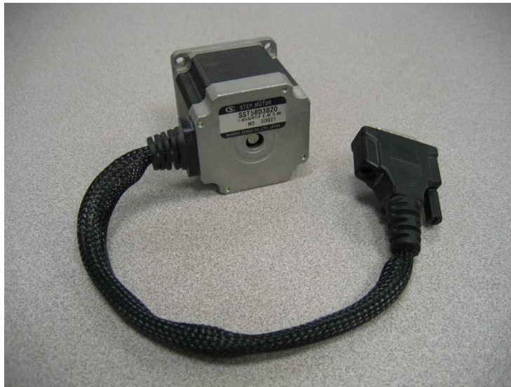
Figure 3.5: An 8 degree/step bipolar stepper motor from Shinano Kenshi Co. Ltd to drive the ER2 robot.
