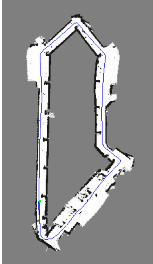
Figure 5.15: Occupancy grid map of Level 3 EA Block of NUS Engineering Faculty after loop closure.
