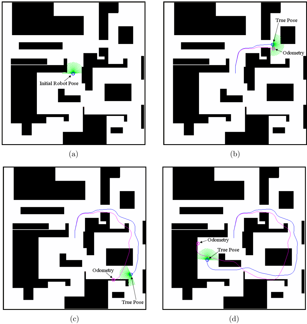
Figure 4.4: Snapshots of the interactive virtual simulator that obtains the true pose of the robot from the user as well as simulates the odometry and sensor measurements. Note that the odometry error grows larger as the robot moves a longer distance.
