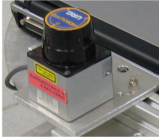
Figure 3.12: URG-04LX laser range finder from Hokuyo Automatic Co. Ltd.
