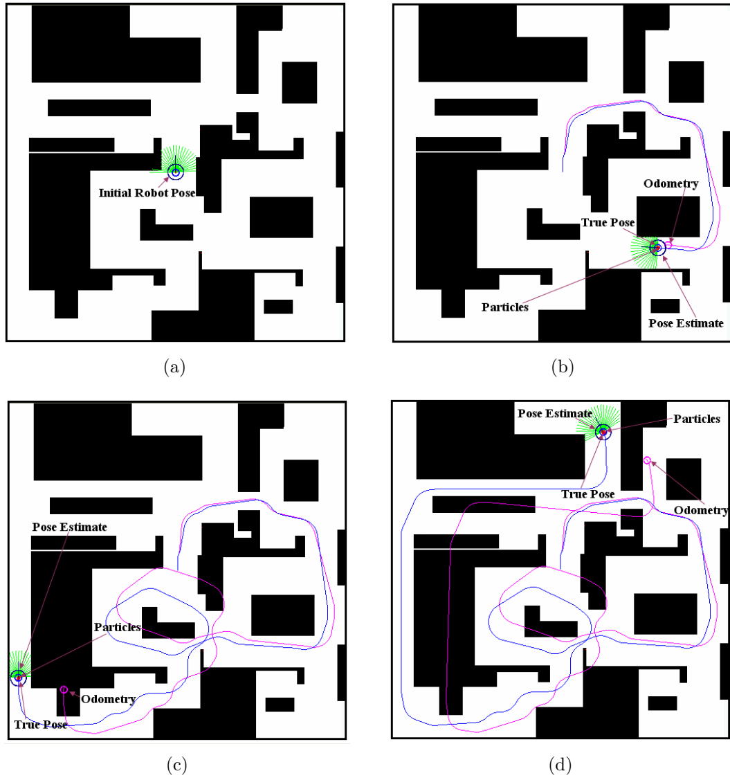
Figure 4.6: Simulation of the local localization problem. The particles are able to give an accurate estimate of the true pose despite the large odometry error.
