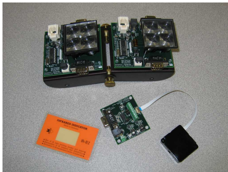
Figure 3.8: NorthStar projector kit (top), detector kit (bottom right) and infrared indicator (bottom left) from Evolution Robotics, Inc. The infrared indicator is used to detect IR light spots since they are not visible to naked eyes.
