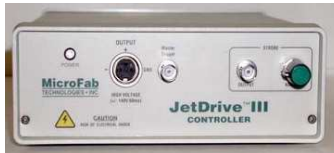
Figure 5.7 Dispenser controller units
