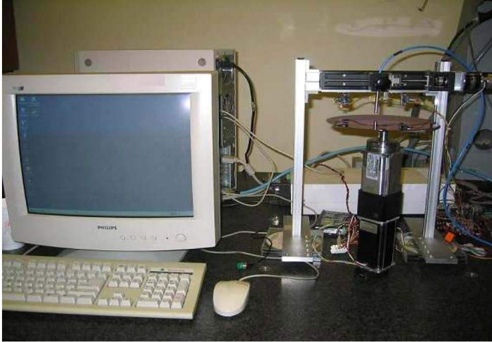
Figure 4.3. The experimental setup for photoresist thickness contour monitoring discussed later. With the availability of the entire thickness contour across wafer, proper assessment and rectification actions can be taken.
