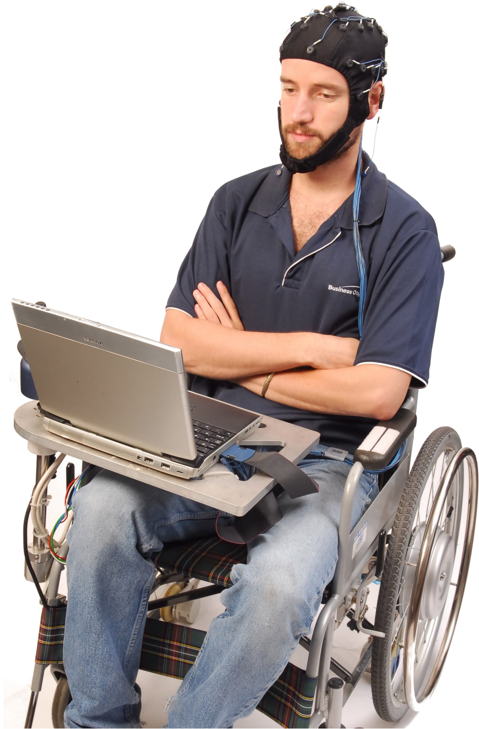
Figure 1.1: Photograph of the prototype Brain Controlled Wheelchair (BCW). The BCW is built on top of a standard powered wheelchair. An EEG cap is used to record the brain signal.
