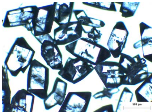
Figure 5-24: Typical micrograph of paracetamol crystals obtained from crystallization experiments. Scale bar represents 500 μm.
