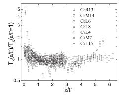
FIG. 3. Log  $T_{\rm K}$  (normalized) inferred from FWHM of 5 K Kondo peak in  $G(V_{\rm SD})$ , as a function of  $V_G$  normalized by the width of the Coulomb blockade charge degeneracy point [ =  $\epsilon/\Gamma$  in the simple model of Fig. 1(a)] for several devices. In the model of Fig. 1(a), a parabolic dependence of log  $T_{\rm K}$  on  $V_G$  is expected. Values of  $\Gamma$  inferred for these devices are, top down, 22.6, 11.5, 18, 3.3, 12.6, 14.2, and 26.8 meV.
