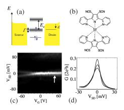
FIG. 1 (color online). (a) Energy level diagram of a typical SET in the Kondo regime. (b) Structural formula of transition metal complex before self-assembly. (c) Map of  $G(V_{SD}, V_G)$  showing transition to Kondo resonance at 5 K. Brightness scales from G = 0 (black) to  $0.3 \times 2e^2/h$ . (d) G vs  $V_{SD}$  at  $V_G = 50$  V [as indicated with arrow in (c)] at (top to bottom) 5 K, 16 K, and 30 K.
