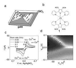
FIG. 2. (a) Diagram of typical single-molecule transistor fabricated by electromigration. (b) structure of **1**, the compound of interest. (c) Cyclic voltammograms showing reversible change in Co ion charge state [26]. (d) Differential conductance of a transistor containing **1**, at 5 K. White corresponds to  $\partial I_D/\partial V_{SD} = 3 \times 10^{-6} S$ . The zero-bias peak in the right-hand charge state is characteristic of Kondo resonant conduction.
