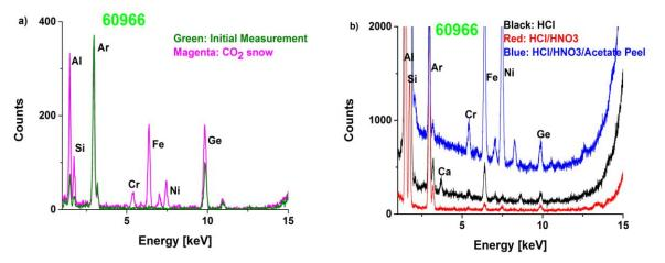
Figure 1: TXRF spectra a) collected with PicoTax after routine UPW/O<sub>3</sub> cleaning (green) and after  $CO_2$  snow cleaning (magenta) and b) collected with S2PicoFox after HCl/H<sub>2</sub>O<sub>2</sub> (black), HNO<sub>3</sub> (red) and acetate peel (blue) treatment.
