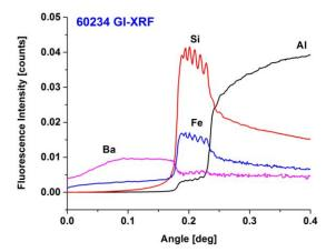
Figure 4: Fluorescence Intensity versus incident beam angle recorded with bench top TXRF for Genesis flight sample 603234.
