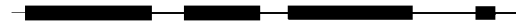
FIGURE 1 Schematic figure showing a typical distribution of fiber segments present some time after the onset of depolymerization. The thin horizontal line indicates the original extent of the polymer. All the ends (eight are present in this realization) are losing material at a constant rate k_{\text{end}} and new breaks are appearing randomly with a rate k_{\text{side}} per unit length of remaining polymer. The kinetics of the resulting depolymerization are analyzed mathematically in this article.
