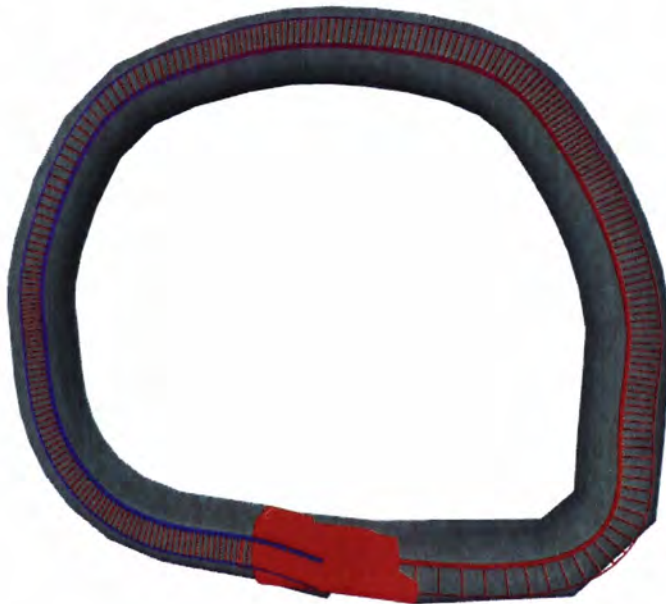
Figure 31: A rod deformed into a closed ring: (a) In perspective and front view, the rod ends do not touch each other; (b) Move one end to another, the mesh of the rod overlaps and causes self-intersection.
