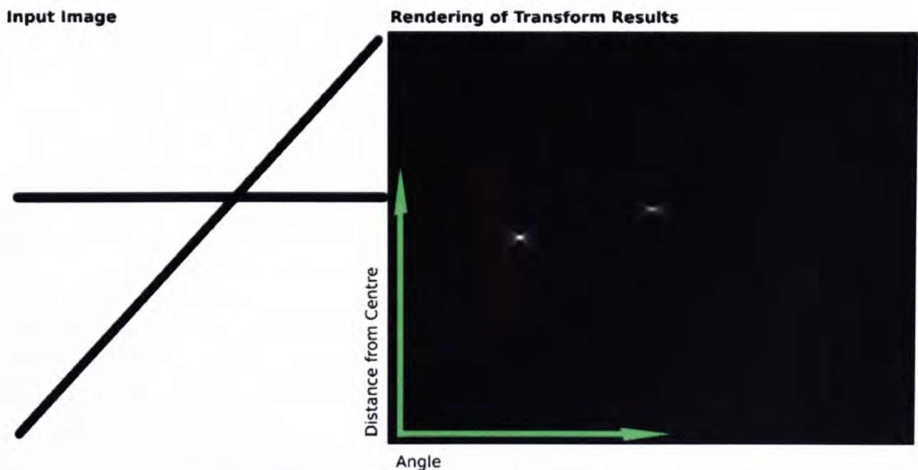
Figure 3.10. Example on Hough transform result
