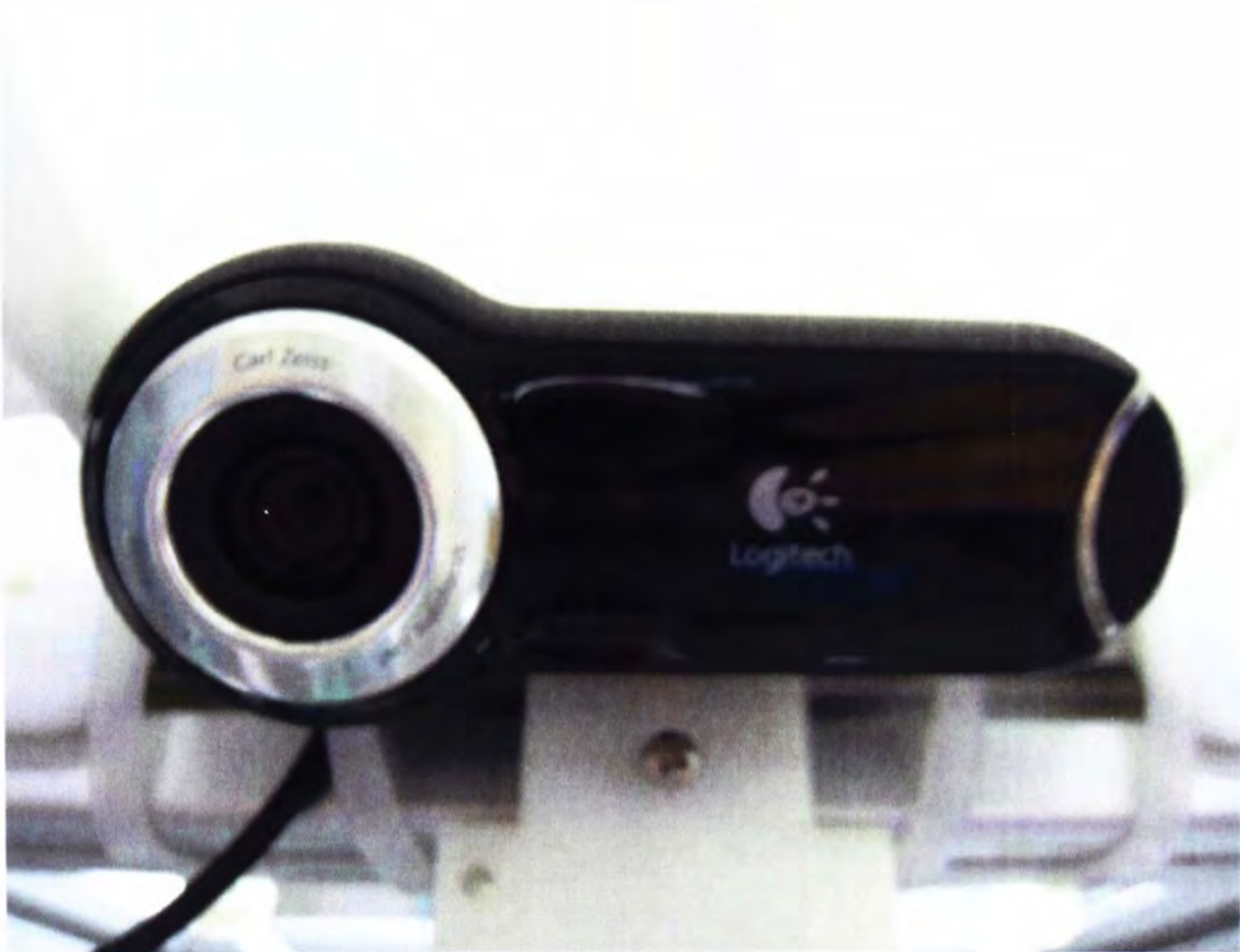
Figure 2.14. Logitech QuickCam Pro 9000 mounted on the Rider
