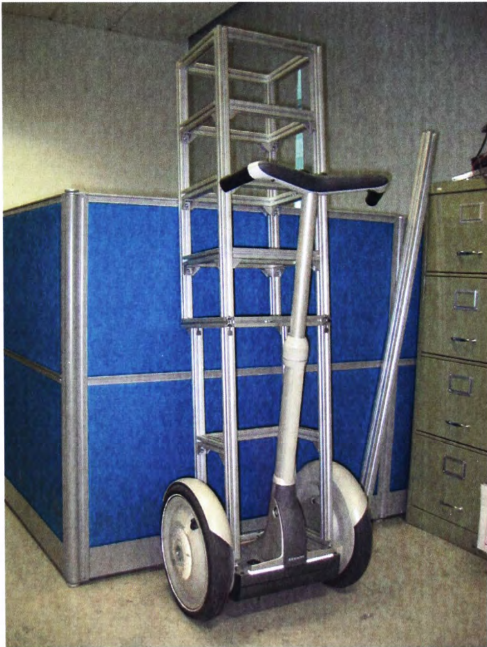
Figure 2.7. Empty profile framework mounted on Segway PT
