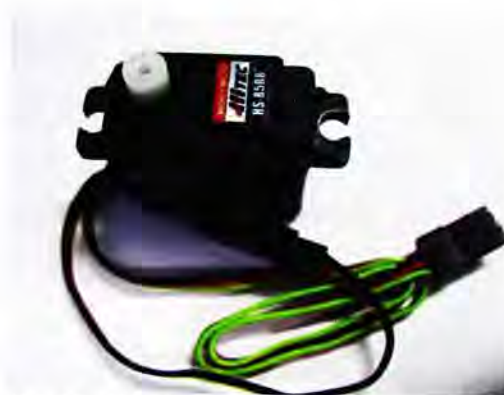
(b) Modified RC servo with wiring for position feedback
