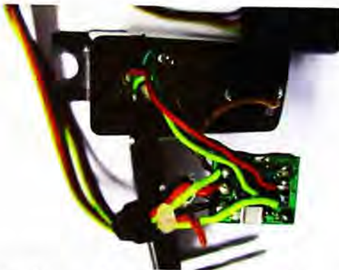
(a) Internal control board, potentiometer and motor of RC servo
