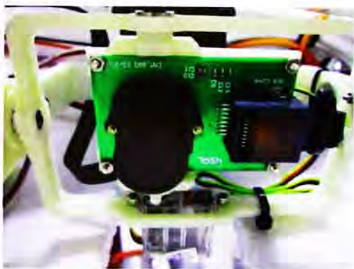
Figure 3.18: Pan-tilt platform installed on foam airplane
