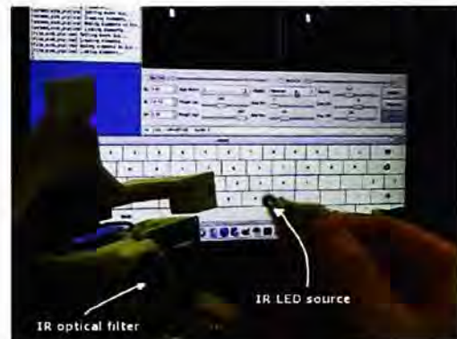
Figure 4.15: Setup for detecting IR point source in indoor
