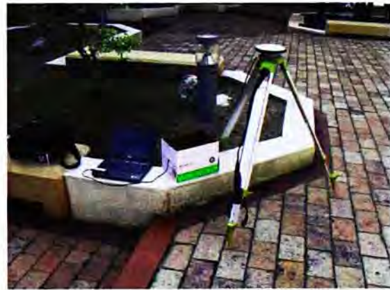
(b) GPS setup for measuring IR illuminator position
