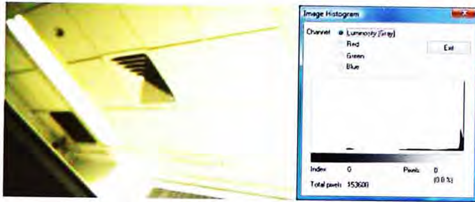
(a) Overexposed image retrieved with large ADC gains
