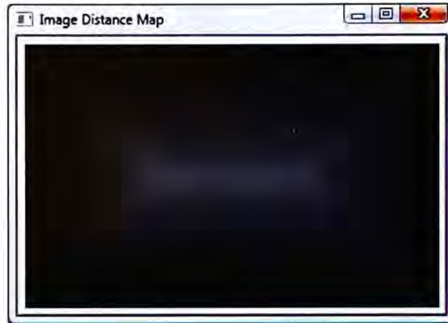
Figure 5.4: Distance map that used for image blending (whiter color indicates larger weight)
