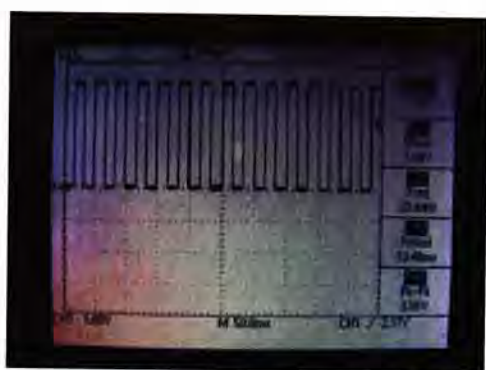
(a) Frame valid signal, valid image frame data at high
