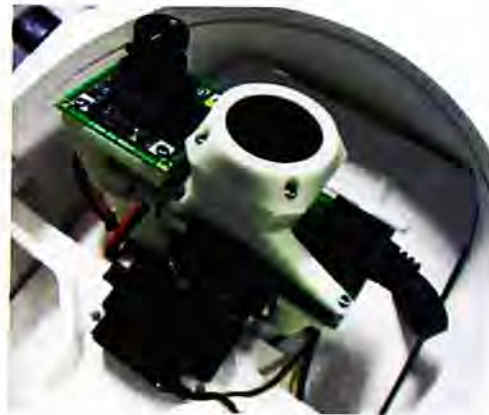
Figure 3.16: Customized micro pan-tilt kit
