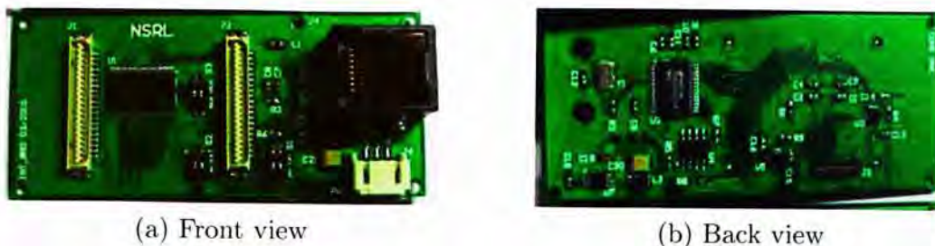
Figure 3.10: Interfacing module of new camera system
