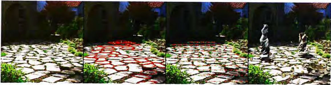
Figure 4.13: From left to right: input photo; extracted cells with local affine transformations estimated; a stable affine transformation field over the cells; and an example photo editing result, where shadow is cast over the analyzed image region.
