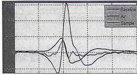
Figure 2.4: Schematic diagram to illustrate the raw data of Air (Blue solid line), Sample (Black solid line) and the calculated Baseline (Red solid line) on the domain.
