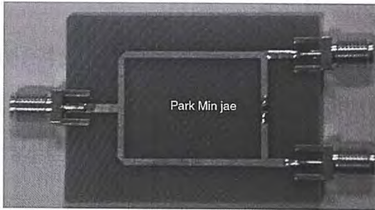
Figure 3.23 Photograph of the modified Wilkinson power divider
