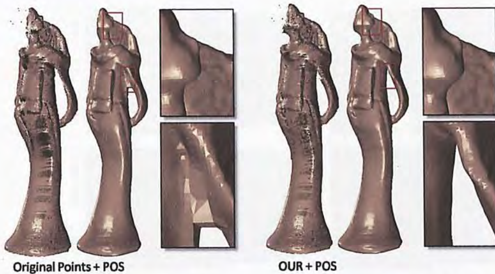
Figure 5.4: A point consolidation and reconstruction of Japanese Lady model: (Left) Raw points and its mesh result. (Right) Points after our point consolidation and its mesh result. The meshes are generated using the POS method.
