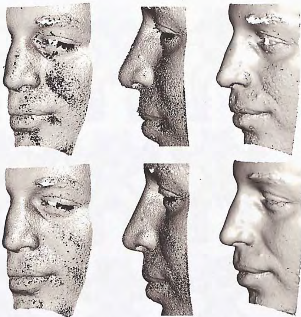
Figure 5.6: Noise removal of a human face model: (Top) The original model and its reconstruction. (Bottom) The model after our framework and its reconstruction. Note that both the point data and the mesh are improved after the treatment. Meshes are generated using INT method.
