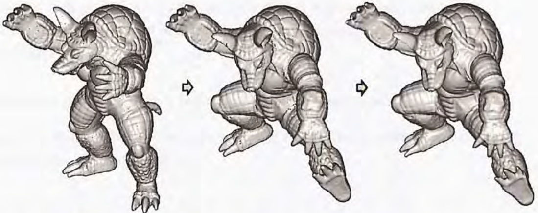
Figure 4.1: Shape modeling on Armadillo model: (Left) The original points, (Middle) points after deformation and (Right) its reconstruction. The meshes are generated by POS method.
