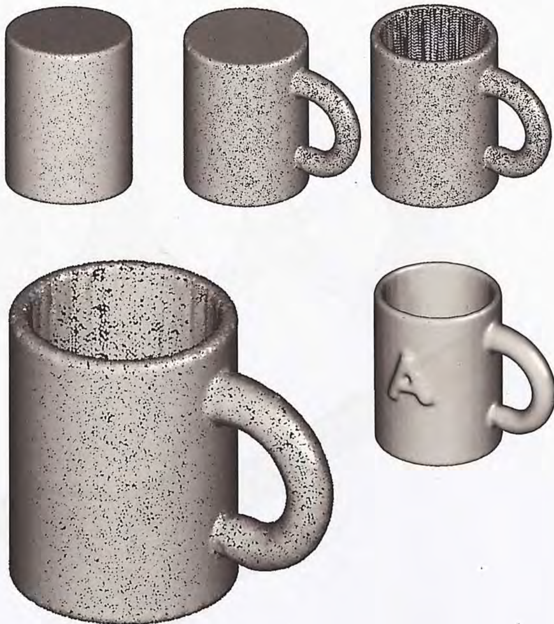
Figure 4.6: Shape modeling on a cylinder: The cylinder is being progressively deformed to a mug. When deforming the container area (First row, right fig.), the large deformation causes the point set to have undesired 'patterns'. The quality is improved by running our consolidation for one iteration (Second row, left fig.). The final mesh result is obtained using POS method.
