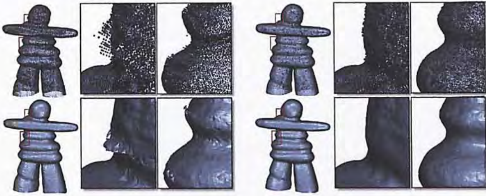
Figure 5.8: Noise removal of Inukshuk model: (Left) Original points and its reconstruction. (Right) Points with our treatment and its reconstruction. It can be seen that our method can remove a small amount of structural noise.
