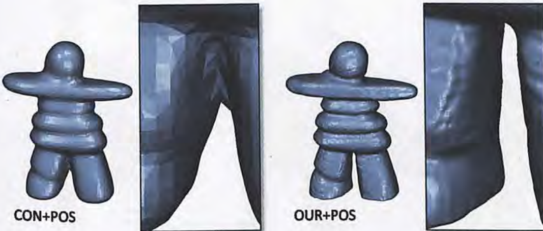
Figure 1.2: The comparison of the Inukshuk model using CON+POS (Left) and OUR+POS (Right). The input after CON has severe drop in the number of points and many details are lost. In OUR method it selectively merges the CON result and the initial input. The structural connectivity is inherited from CON while the details are still preserved.
