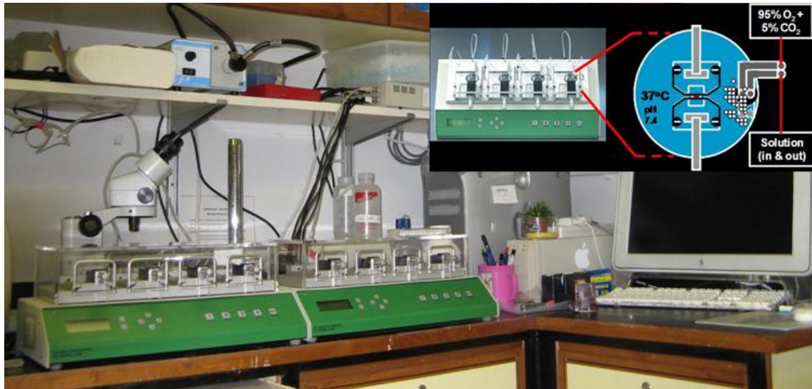
Figure 8. Myograph setup for measuring isometric forces generated by smaller arteries such as the rat femoral artery.
