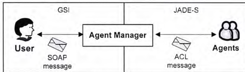
Figure 6-2: Message exchange in MGS
