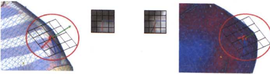
Figure 3-26: The upper row illustrated the region covered by the feature descriptor centered from an anchor point. The bottom row illustrated the feature descriptor of the anchor point. Blue region indicated the searching region and best descriptor matching of the template.
