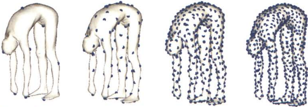
Figure 4-3: Sample points defined by the Farthest Point Sampling on example 2. Number of sample points = 10, 100, 200 and 500 from left to right.
