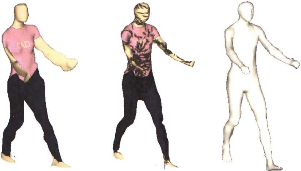
Figure 3-19: Surface fitting result (middle) of a posture aligned template (left) to input model (right) by generic approach. Smoothness distracted in black region, arm wrongly mapped to opposite side.
