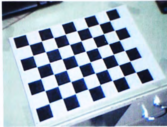
Figure 3.3 Template for camera calibration with 30x30mm grid
