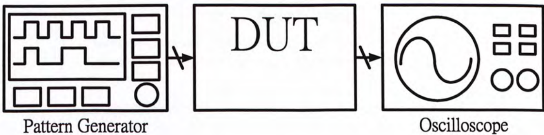
Fig. 8.4 Block diagram of measurement setup
