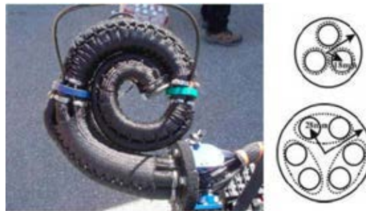
Figure 1-5 OctArm: OctArm V Prototype (left); Muscle Configuration (right) [37]
