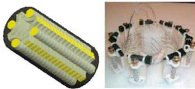
Figure 1-7 Octopus Arm: Muscle Configuration (left); Prototype (right) [47]
