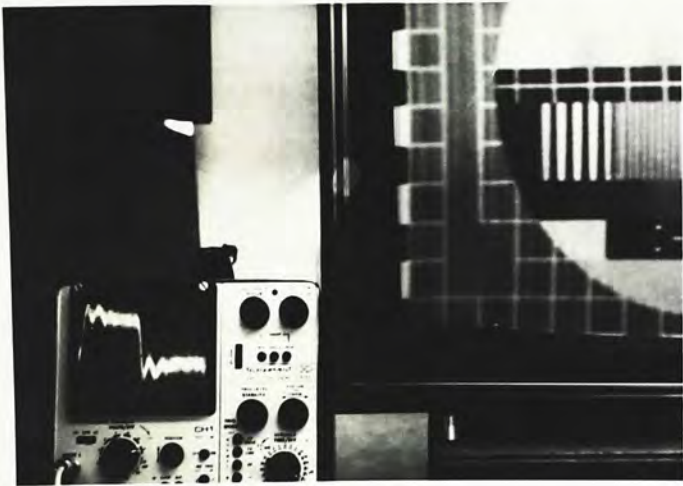
Figure 2-4-4. Picture after cancellation with incorrect time delay-longer in time.
