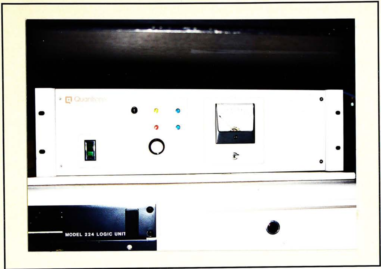
Figure A1-pIII The RF driver unit for the acousto-optic mode-locker. The output frequency is 41 MHz.
