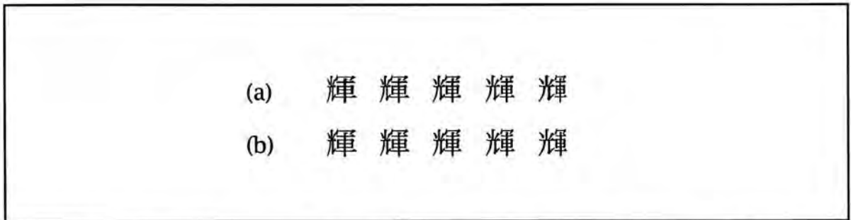
(a) Unhinted images (60x60) of radicals scaled from -30% to +30%. (b) Hinted images (60x60) of radicals scaled from -30% to +30%
