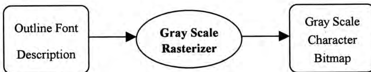
Figure 5.1 Generation of gray scale font using gray scale rasterizer
