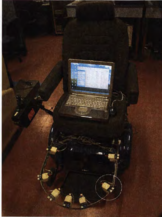
Figure 3.1: The wheelchair platform with 7 ultrasonic sensors in the front(Circled).
