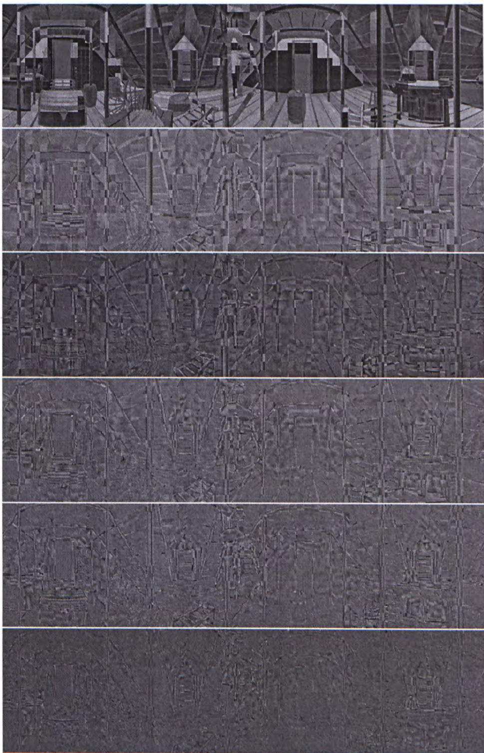
Figure 6.1: The first 6 tiled eigenimages ( Y channel) of 'attic'.
