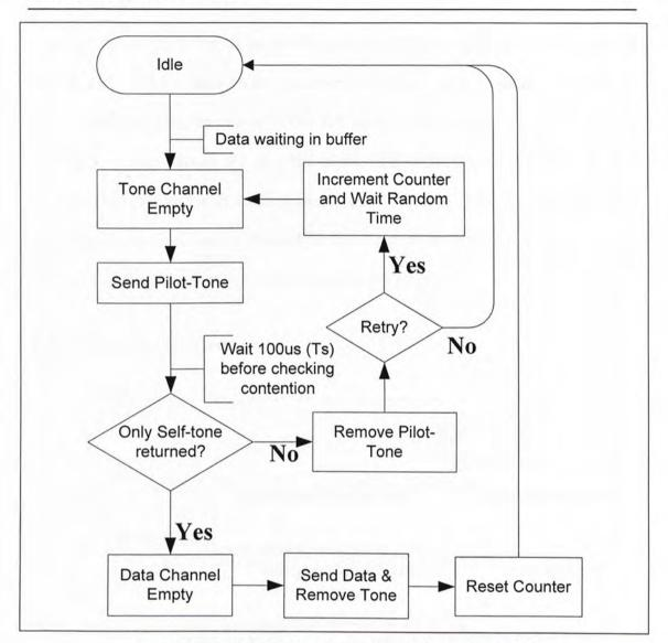
Figure 3.2 CSMA/CA protocol using Pilot Tone on PON
