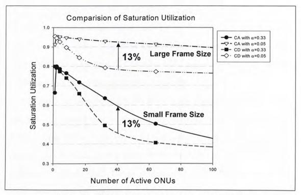
Figure 3.9 Effect of Network size on Saturation Utilization
