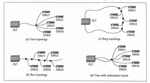
Figure 1.2 Typical PON Architecture
