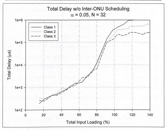
Figure 4.13 Total Delay without using Inter-ONU Scheduling
