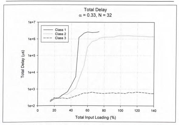
Figure 4.12 Total Delay for 3 different classes of service for  $\alpha = 0.33$
