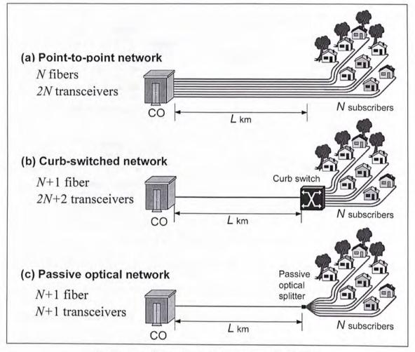
Figure 1.1 Three Types of Optical Access Network
