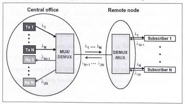
Figure 1.4 WDM PON Architecture
