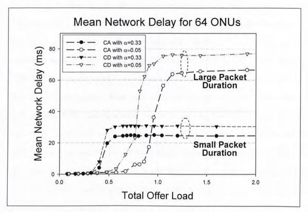
Figure 3.10 Effect of loading on delay
