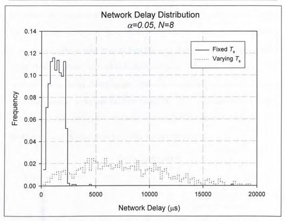
Figure 4.6 Network Delay Distribution during Saturation over 1 second
