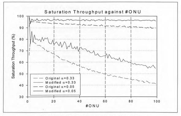
Fig. 4.3 Saturation utilization against Network Size
