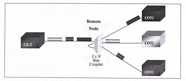
Figure 3.1 Physical Network Connection
