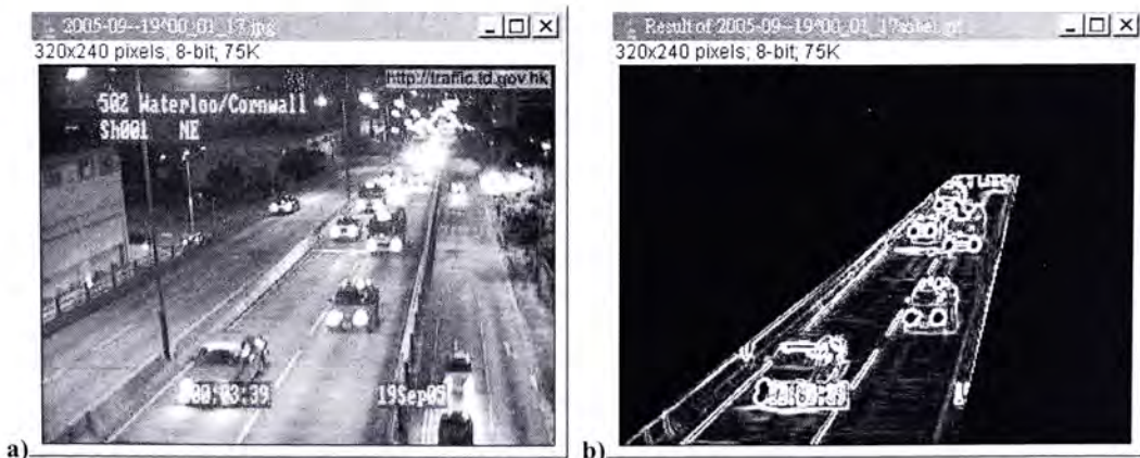
Fig. 4.8 Image under night condition (a) Grayscale image (b) Edge image with circular edges rather than horizontal edges
