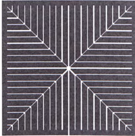
Figure 2-7 Patterned ground shield for spiral inductor
