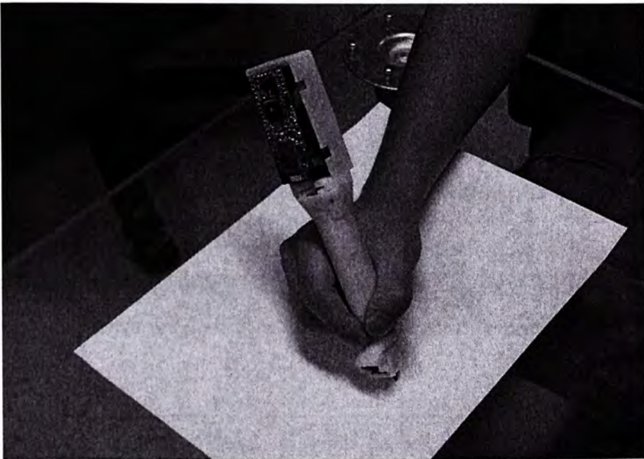
Figure 8.12: Experiment setup for Digital Writing Instrument with MAG- \mu IMU
